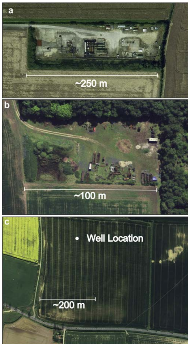
Figure 13. Examples of wells locations taken from UKOGL imaged with Google Earth, illustrating range of surface manifestations of UK onshore wells: (a) cleared area of land with appearance of being a maintained well pad; (b) cleared area of land with appearance of poorly maintained and potentially disused well pad. (c) Location of well drilling in which no well pad or machinery is visible.
