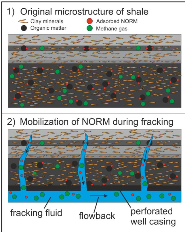
**Figure 1:** Schematic diagram of NORM in shales.
